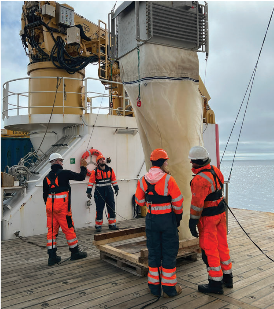
Plate 179. ‘Mammoth net’ being deployed onboard the SDA 8 December 2023. The net is carefully lowered to a designated depth, before being slowly recovered. During the ascent, a pressure sensitive mechanism will open and close up to ten-separate nets at different depth ranges. This enables the unique biota of the Antarctica water column to be recorded as it changes with depth.
