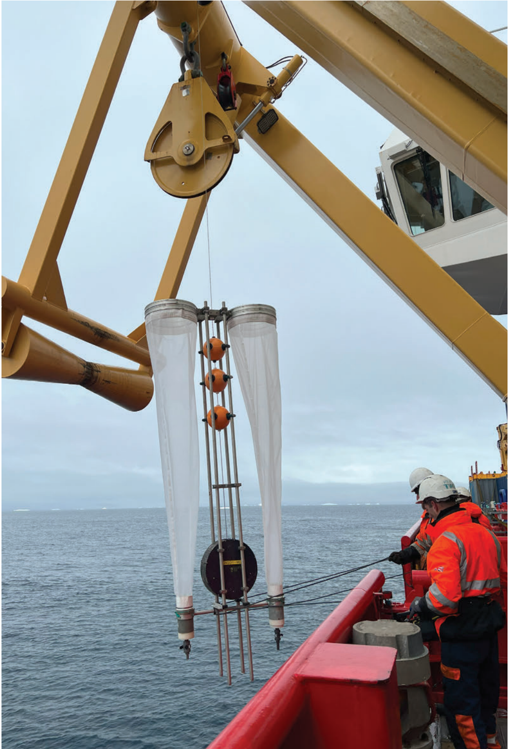
Plate 180. 'Bongo net' being deployed onboard the SDA 8 December 2023. This net is typically lowered to a depth of approximately 200m, before being slowly recovered, sampling the organisms of the Antarctic waters. Through repeat samples and careful extrapolation, an estimate may be made of the total biomass in the Antarctic waters.
